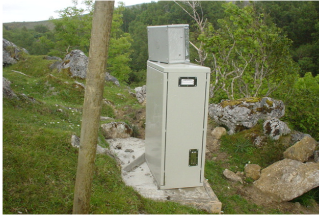
Flood level recorder at the Cladagh River sink, Marble Arch Caves
